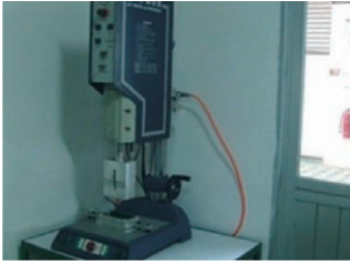
Ultrasonic Welding for Sealing Plastic Case
