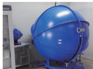
Integrating Sphere (for Testing LED Luminous)
