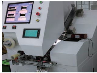
3 in 1 Auto inspection machine (Flatness/ Visual/ Taping)
